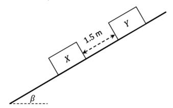
The coefficient of friction between X and the plane is  $\frac{1}{2}$  and the coefficient of friction between Y and the plane is  $\frac{2}{5}$ . The blocks are released from rest.
