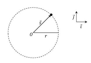
The motion of the car may be modelled as horizontal circular motion around centre O, with radius r and constant angular speed  $\omega$ , as in the diagram above.
